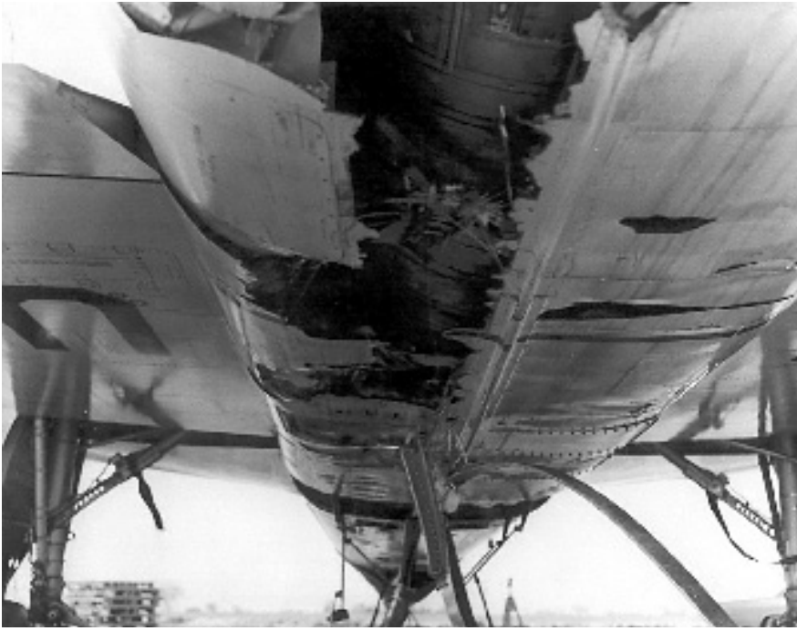
The undercarriage of the F-106 was damaged in the landing near Big Sandy, Mont. It could have been a lot worse.
