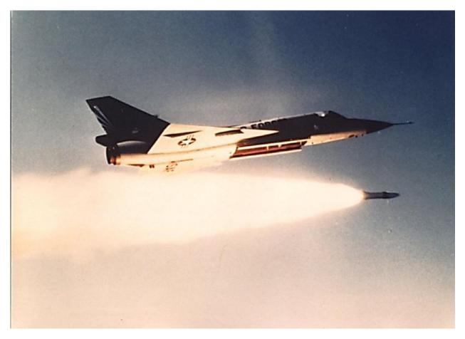
F-106A of the 49<sup>th</sup> FIS Griffiss AFB, NY Firing an Air-2A Genie Nuclear Rocket
