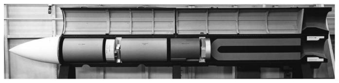
GAR-9 mockup displayed in 1959 opened to depict internal components. Major subassemblies, from left to right: HE warhead, angular rate sensor and control units, electronics unit, umbilical unit, rocket motor (National Archives via Dennis R. Jenkins)
