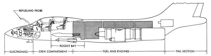
F-101B cutaway depicting the weapons configuration when employing the AIR-2 (USAF via Ryan Crierie)
