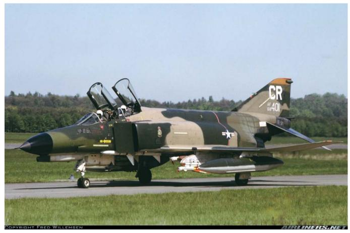
A USAFE Soesterberg-based F-4E armed with four AIM-4D missiles in September of 1973 (Fred Willemsen) Dassault Mirage IIIS
