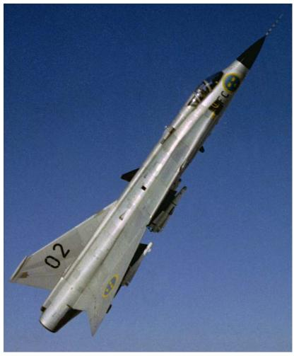
The first J-35F, armed with Saab Rb.27 (underfuselage) and Rb.28 (underwing) Falcon AAMs (Saab AB)
