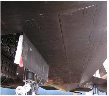
YF-12A tandem missile bays located in the starboard chine; F-12B bays would have been similarly arranged (Sean O'Connor)
