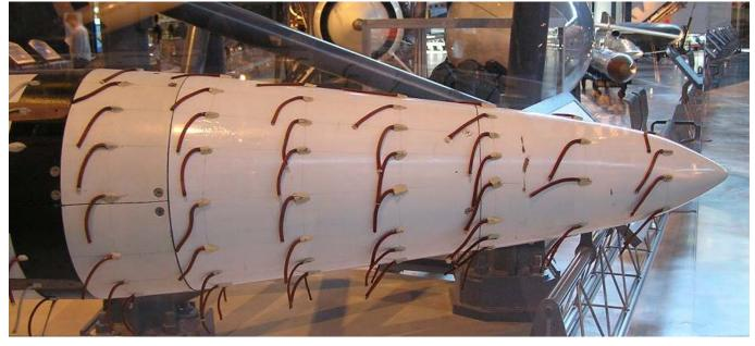
The AGM-76A employed a revised nose profile housing a passive radar seeker (Sean O'Connor)
