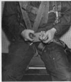
Fig. 6. Shoulder harness loops are installed on lap belt link.
