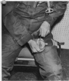
Fig. 5. Aircrew inserts Gold Key into buckle.
