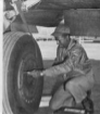
Highly thought of B-57 crew chief, Sgt Jimmie K. Armwood, checks tire pressure, B-57A.
