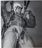
When the lowering device is needed, the snap and buckle is removed from the storage pocket.
