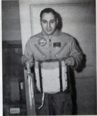
150 feet of lanyard is stored inside the lowering device container. The last 25 feet of the lanyard is yellow to serve as a warning.
