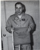
The CPU-10/P lowering device is packed in a foam padded container and replaces the standard parachute back pad.
