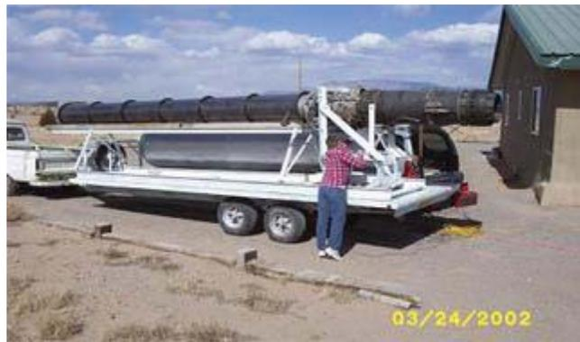
**Figure 7 – J85-5 Mobile Test Rig**
