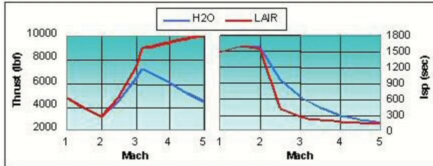
**Figure 3 – Representative J85 Engine Data for Maximum Thrust Trajectory**
