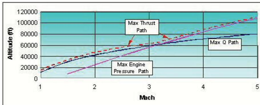
**Figure 2 – Maximum Thrust Trajectory Profile**
