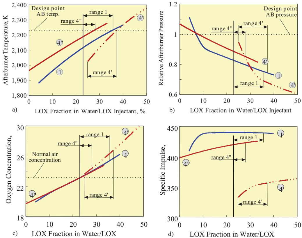
**Figure 5 - Combustion parameters as a function of LOX fraction in water/LOX injectant for selected MIPCC engine zoom maneuver operational modes 1, 4', and 4''(see Figure 4).**
