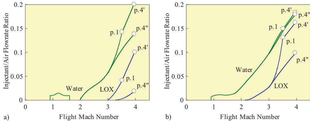
**Figure 6 – Relative water/LOX ratio for simulated turbojet (a) and turbofan (b) engines.**
