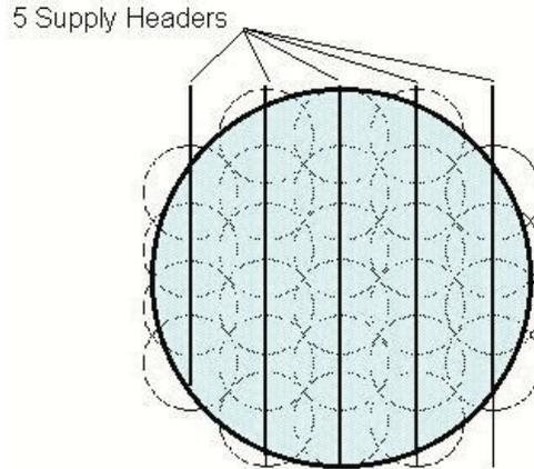
**Figure 8 – MSE Injector Configuration: 5 Headers, 26 injectors**
