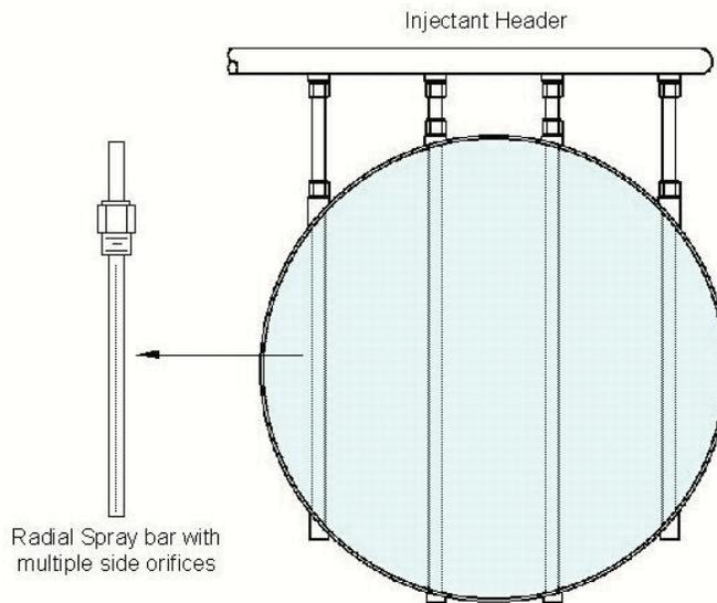
**Figure 9 – HMX Injector Configuration: 4 Spray Bars, Side Drilled Spray Orifices**
