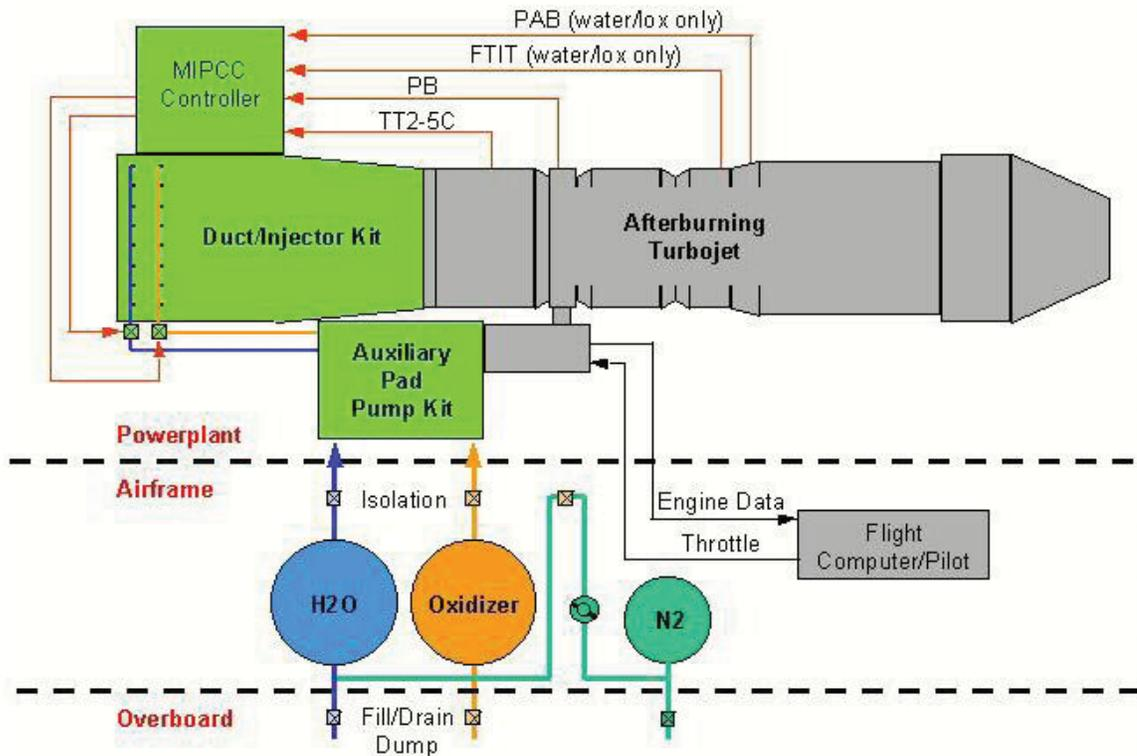
**Figure 10 – MIPCC System Schematic**
