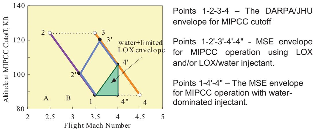
**Figure 4 - Flight envelopes for the end of zoom maneuver**
