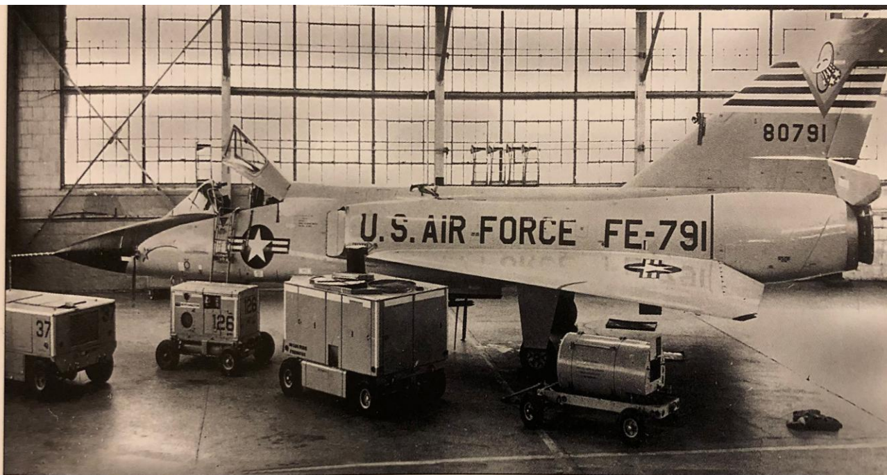
With a 94th FIS Six in the background, this 1960 photo shows some of the specialized AGE equipment needed. From left to right are: M32A-13, MC-11, MA-3, and a LOX cart. When the IRST was added, a similar cart was used to service the system with liquid nitrogen. (USAF via El Mason)
