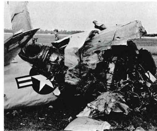
During a low go-around from an SFO the engine failed. The pilots apparently kept their altitude and bled off the airspeed. The T-bird faltered and fell off on one wing. Neither pilot attempted to eject.
