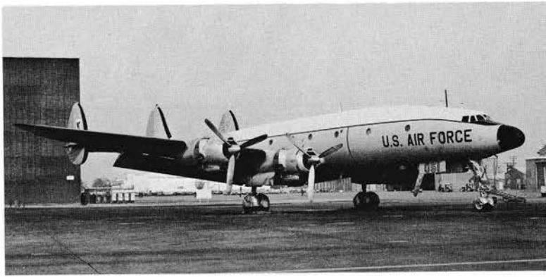
The G-Model. This is the basic transport model and closely resembles the original commercial version of the Lockheed Constellation. It is the primary support aircraft used for local transition flights, training, flight checks, and moving personnel and equipment.
