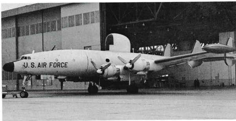
The D-Model. The most familiar, basic surveillance model with its upper and lower radome transceiver radar antennas. Its "manual" search and control function is presently giving way to major automatic equipment modifications, and is slated for operation with reserve forces in Florida. The Q-Model looks just like the "D" from the outside but has been internally modified for specific requirements peculiar to special surveillance missions.
