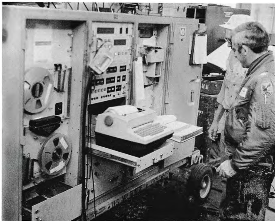
The USM-185 checks out aircraft wiring before the electronic equipment is reinstalled. Computer tapes roll, circuits hum, and a typewriter prints out problem areas.
