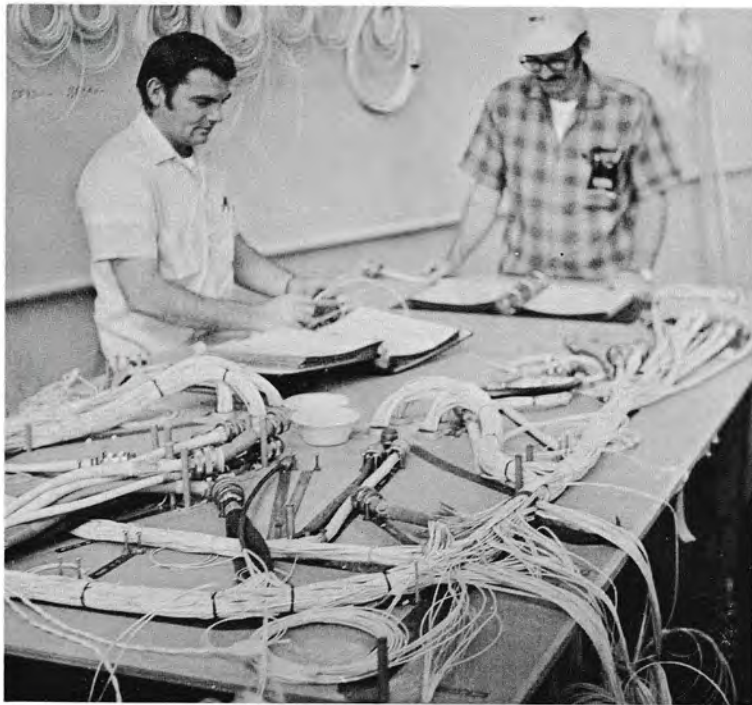
Technicians work around "bread boards" that simulate the F-106 cockpit, building new wiring harnesses out of "micro" wire. This modification does away with the old splices and repairs, and reduces the overall size of the wiring bundles.
