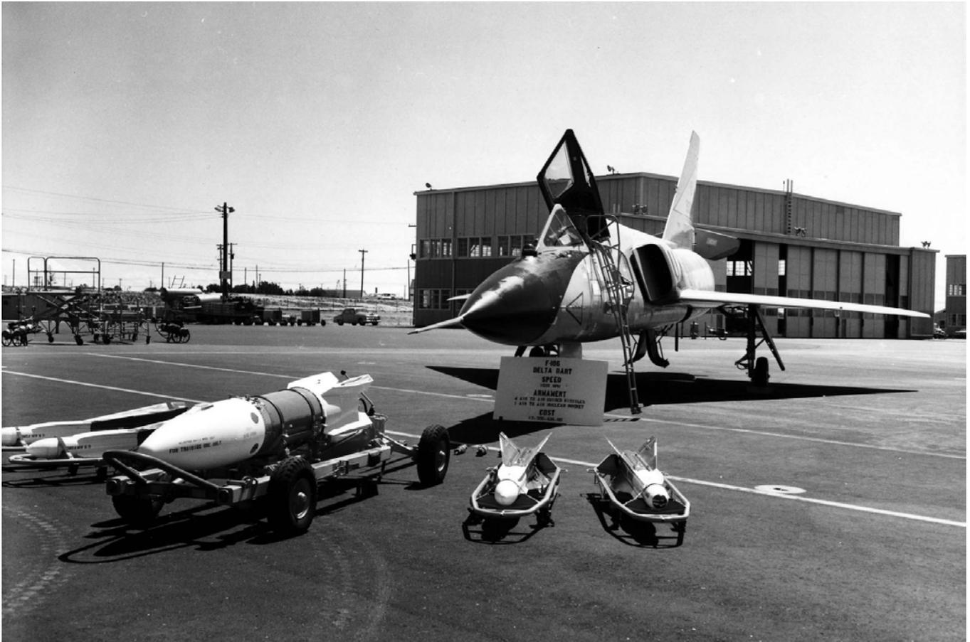
F-106A displayed with a complete weapons load consisting of two GAR-3A and two GAR-4A missiles and a single Genie nuclear rocket (USAF Museum)
