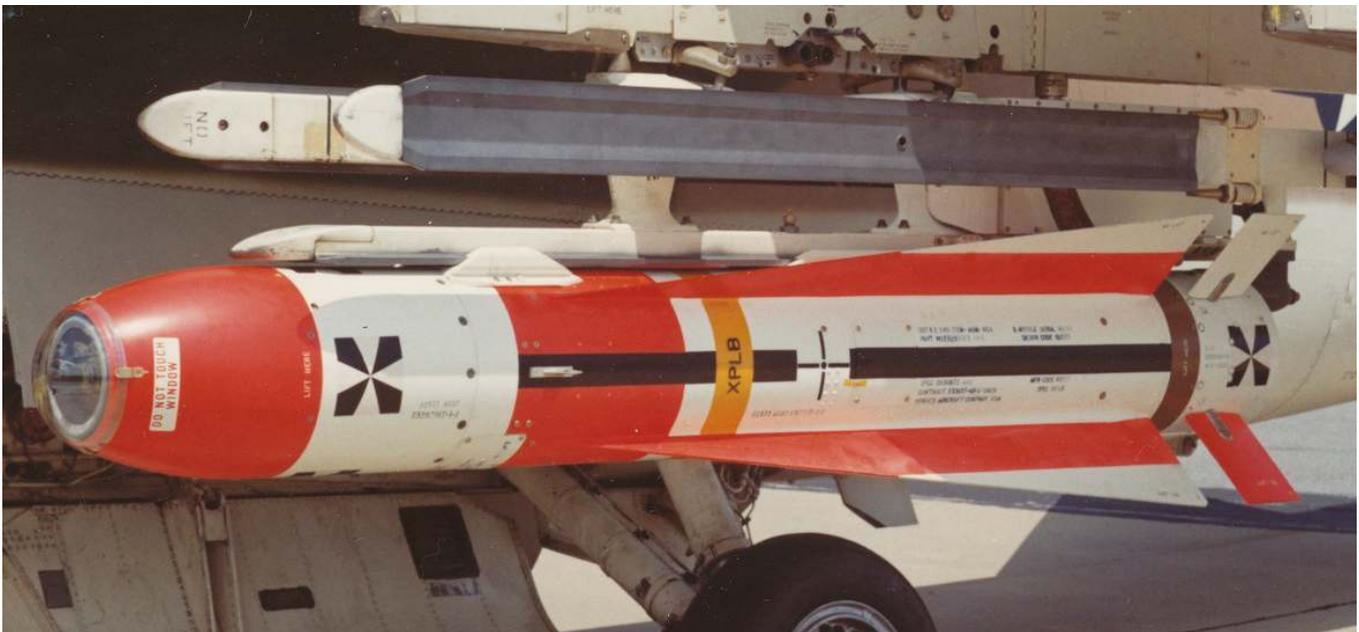
**AGM-65A test round illustrating the retention of the Falcon missile planform (USAF via Ryan Crierie)**
