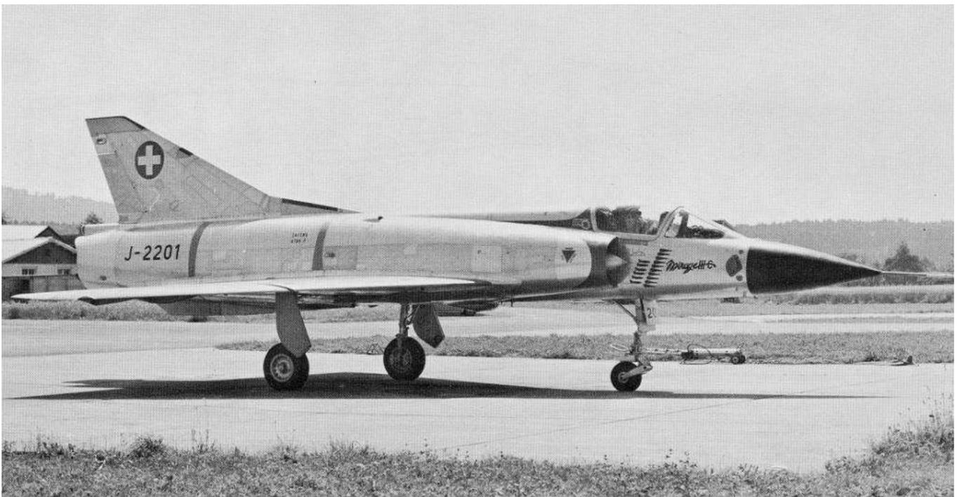
Mirage IIIC J-2201, used in HM-55 separation trials (Swiss Air Force)
