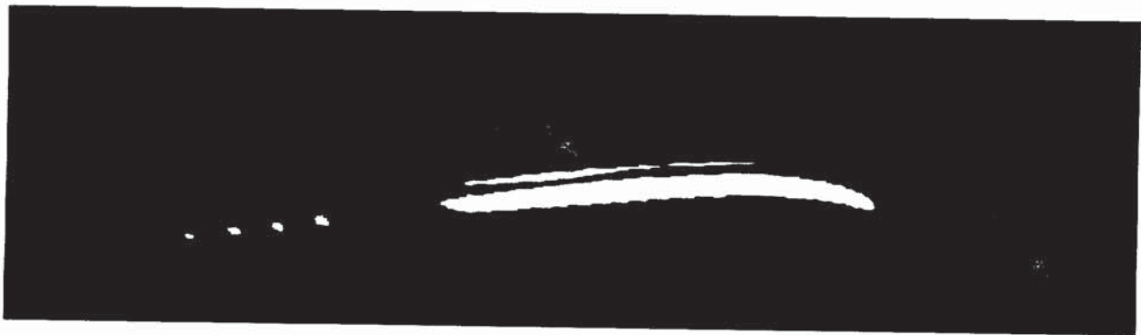
Figure 19(a). – View of vortex at lightsheet position of 88^\circ , \alpha = 11^\circ , \beta = 0^\circ , 30^\circ vortex flap.
