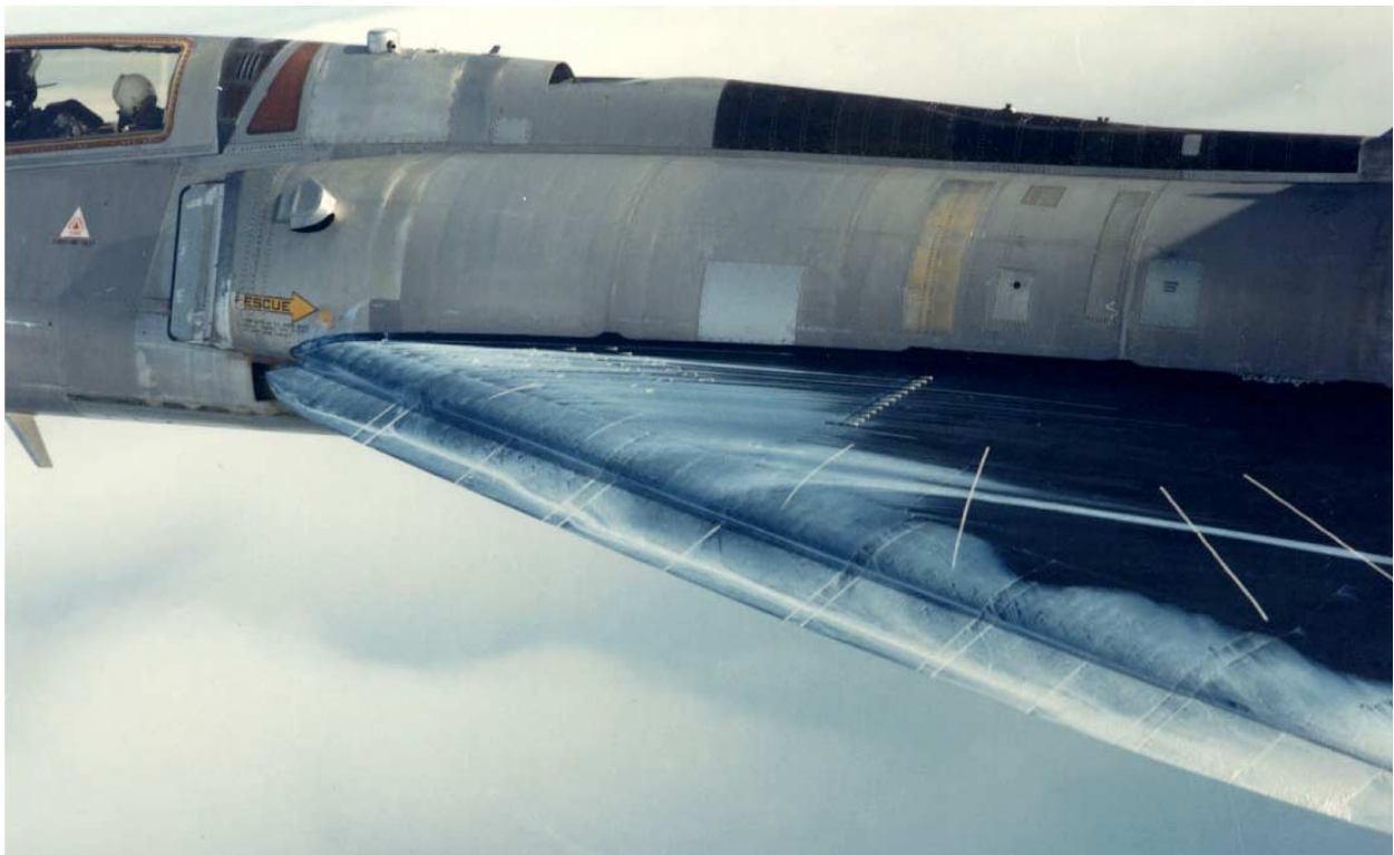
Figure 13. – Surface oil flow patterns, \alpha = 13^\circ , 30^\circ vortex flap.
