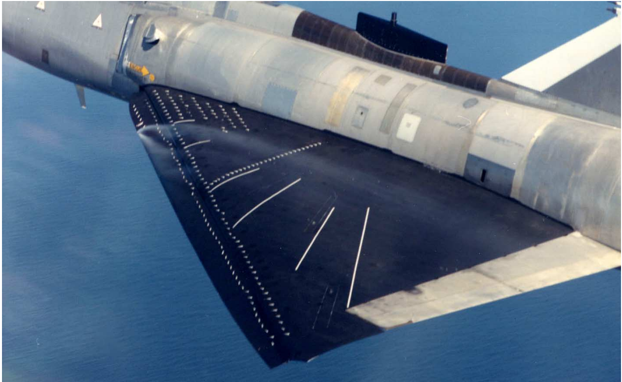
Figure 7. – Daytime smoke, \alpha = 9^\circ , 30^\circ vortex flap.
