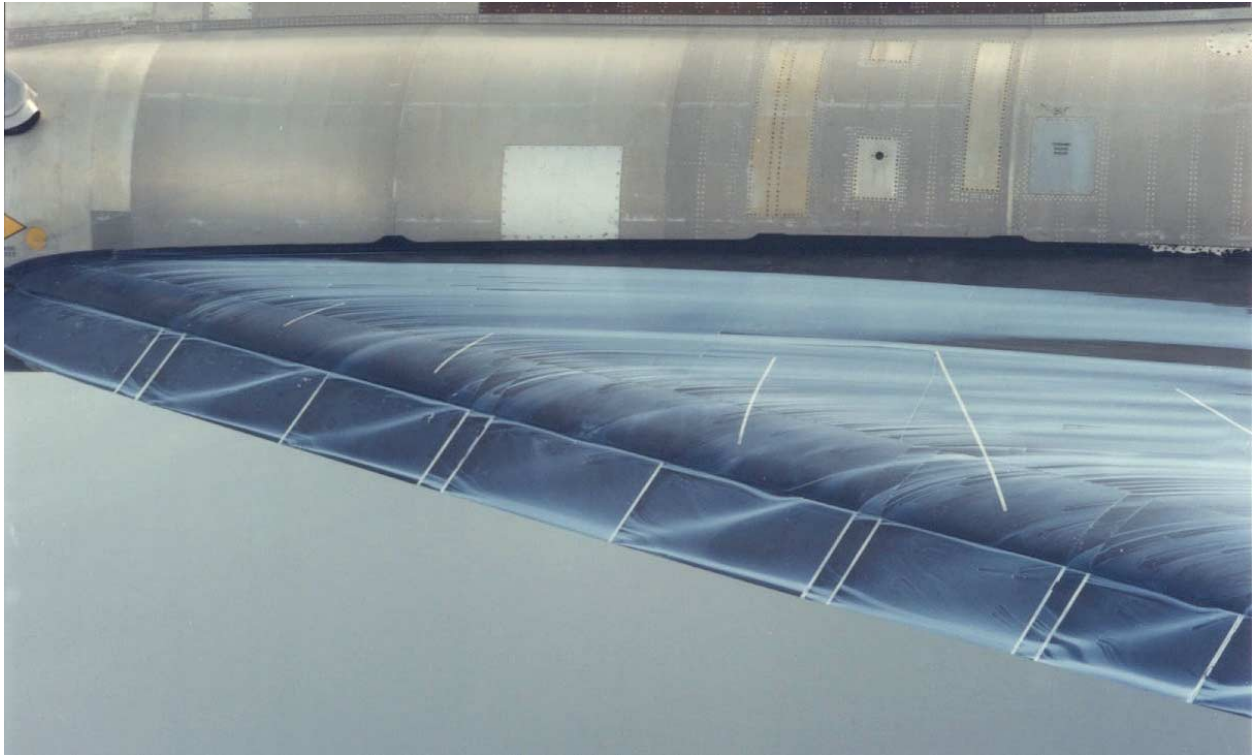
Figure 22. – Oil flow patterns, \alpha = 11^\circ , 40^\circ vortex flaps.
