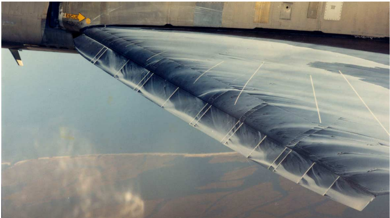
Figure 25. – Oil flow patterns, \alpha = 13^\circ , 40^\circ vortex flaps.
