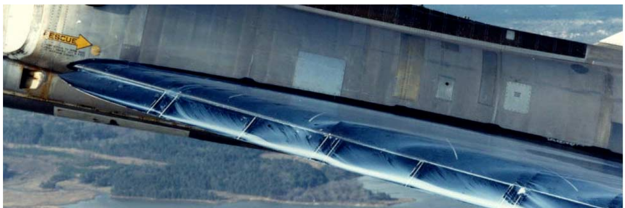
Figure 28. – Detail of forward sections of the vortex flap, \alpha = 15^\circ , 40^\circ vortex flaps.
