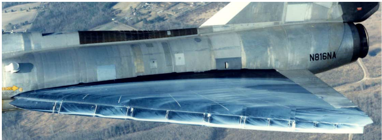
Figure 27. – Oil flow patterns, \alpha = 15^\circ , 40^\circ vortex flaps.
