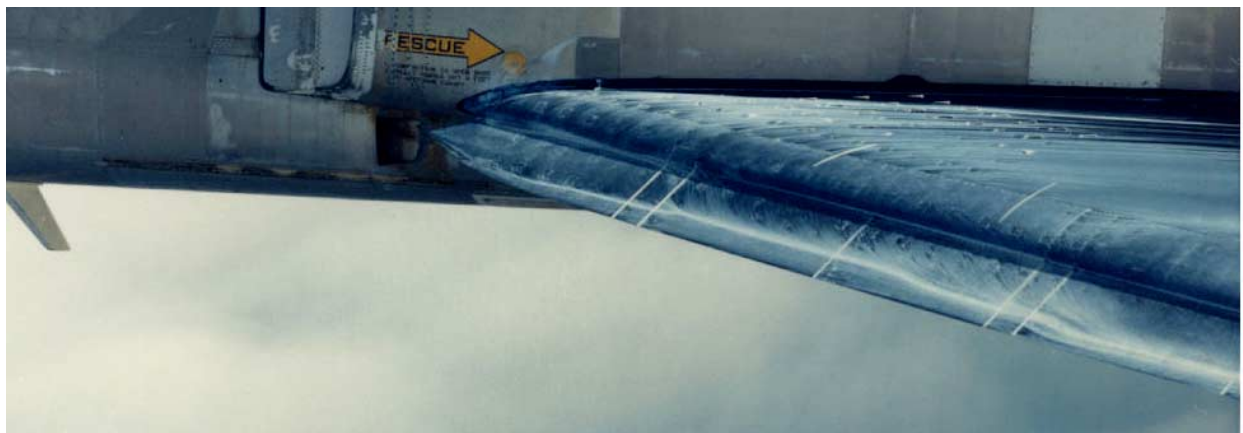
Figure 14. – Detail of apex area, \alpha = 13^\circ , 30^\circ vortex flap.
