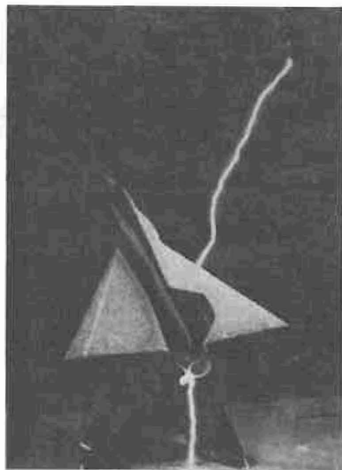
Fig. 16. Strike attachments to leading edge of left wing with exit from engine exhaust area of scale model. Rod electrode positioned equidistant from nose boom and right wing tip; model pitched 45^\circ nose up; positive polarity electrode.
